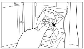
7. Fit the stapler unit all the way to the machine, until the green lever goes up.
